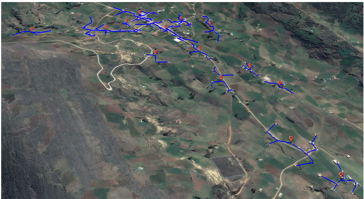
Figure 32 Zoom in land projection of a village electrified with 14 microgrids and several SAS for the Base Case Scenario
